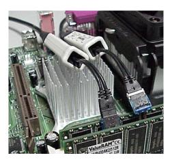
Figure 20: Circuit board with Tip-Clip assemblies
